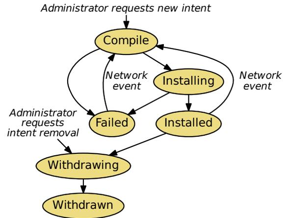
**Figure 1: Intent compilation and installation of a single intent within a generic intent state machine model. Intents (and their low-level updates) are impacted by administrator events (e.g., requesting a new intent be installed, withdrawing an existing intent) or by network events (e.g., topology change).**
