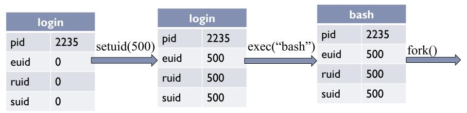
After the login process verifies that the entered password is correct, it issues a setuid system call.
