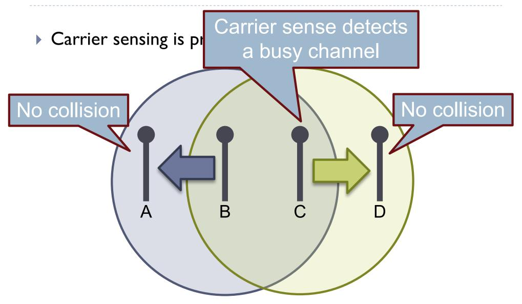
□ ■ Garrier sense can erroneously reduce utilization Data link.
