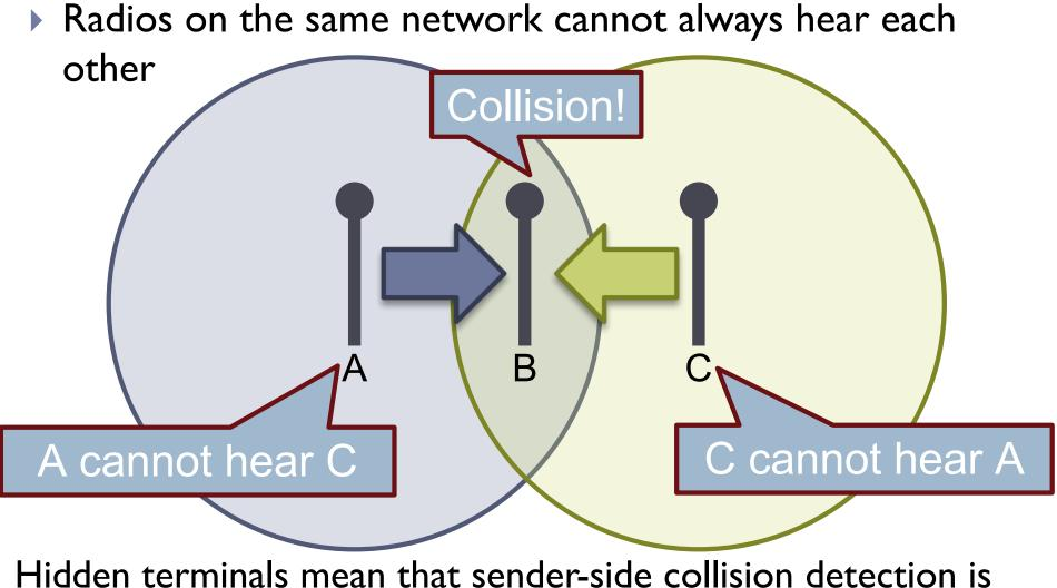
Hidden terminals mean that sender-side collision detection is us<sup>4</sup>eless
